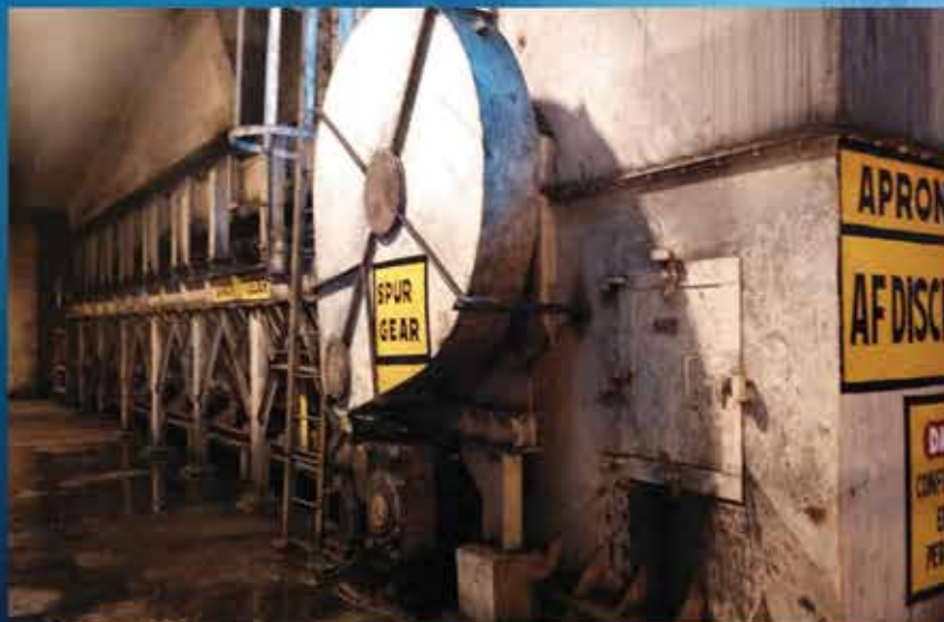
Apron Feeder - Bottom of Wagon Tippler Complex
