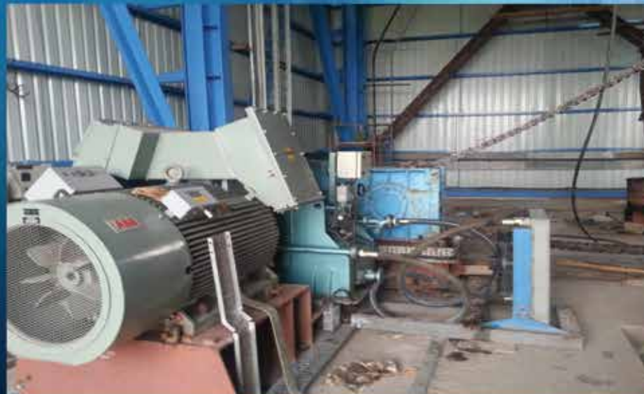
Drive Assembly for Rotary Breaker
