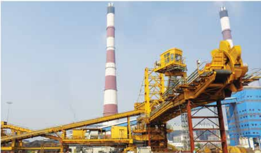
Stacker Reclaimers - Erected at Jharsuguda, Odisha, India
