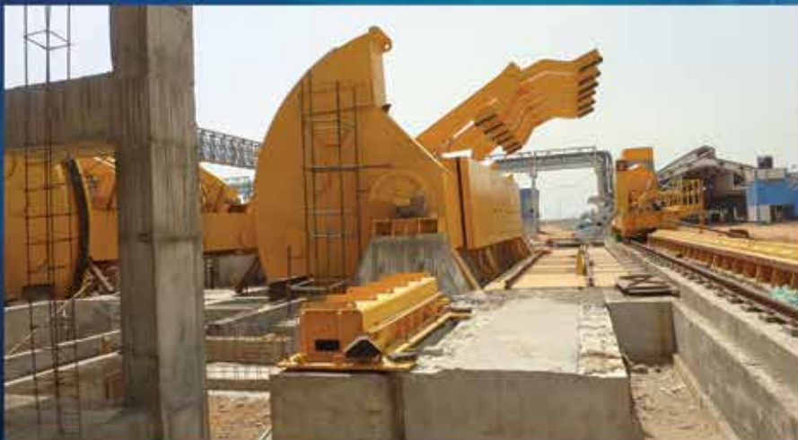
Wagon Tippler with 6 pause and 3 Clamping Cylinder
