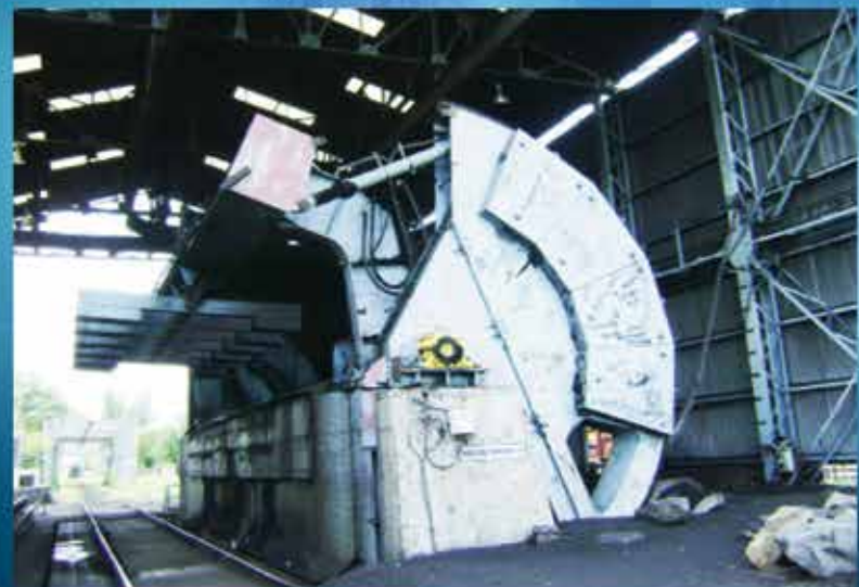
Hydraulic Wagon Tippler with 6 Clamping Cylinder with upper holding beam
